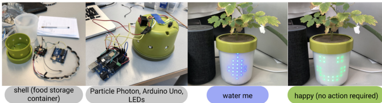
Figure 1: Images of PlantBot design. From left: Shell, electronics, water drop emoticon, and happy face emoticon. 9
