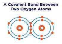
Notice in the diagram above how four electrons are being "shared" between the two Oxygens. This is how a covalent bond looks like when two nonmetals are bonded together.
