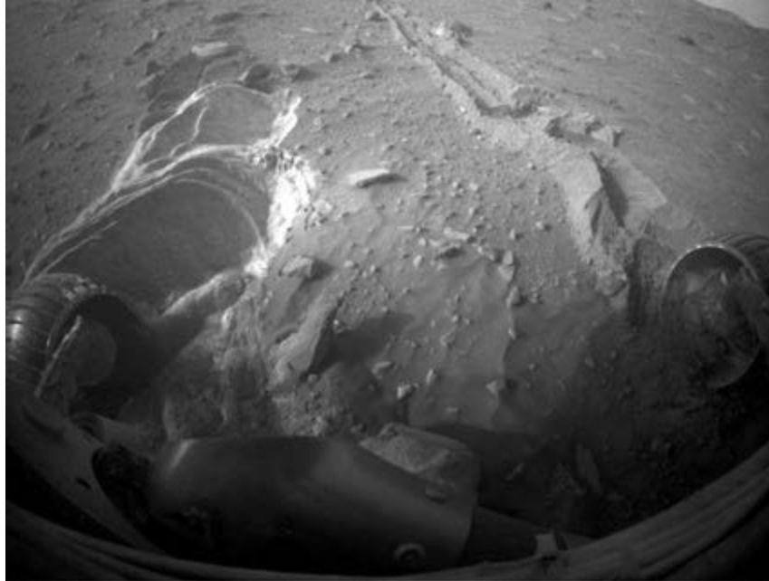
Figure 30: Final images from the spirit rover after it got stuck in a sand trap [9]
