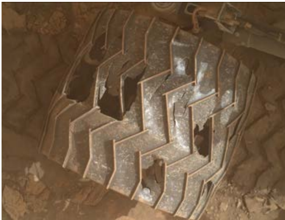
Figure 31: Wheels of Curiosity rover damaged due to rugged terrain [10]
