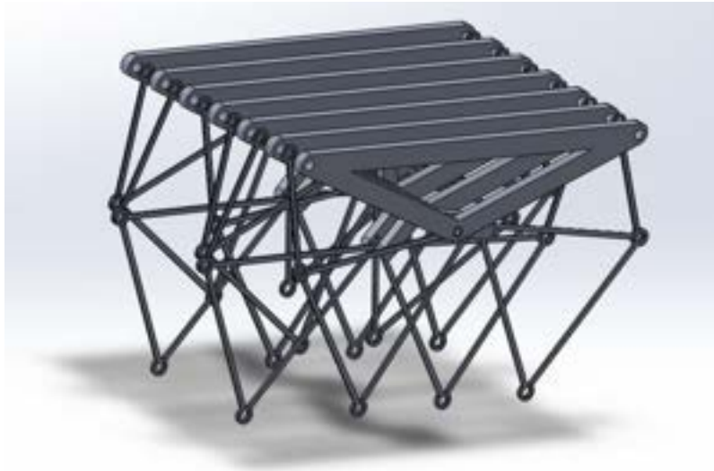
Figure 23: All main frames added to assembly
