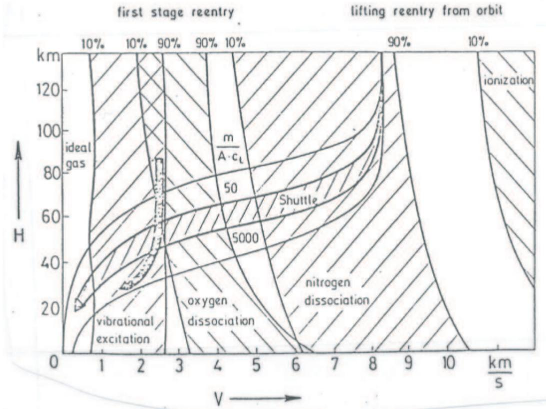
Fig. 1.1 - Map of hypersonic flight regimes (velocity on the x-axis, height in atmosphere on the y-axis). [2]
