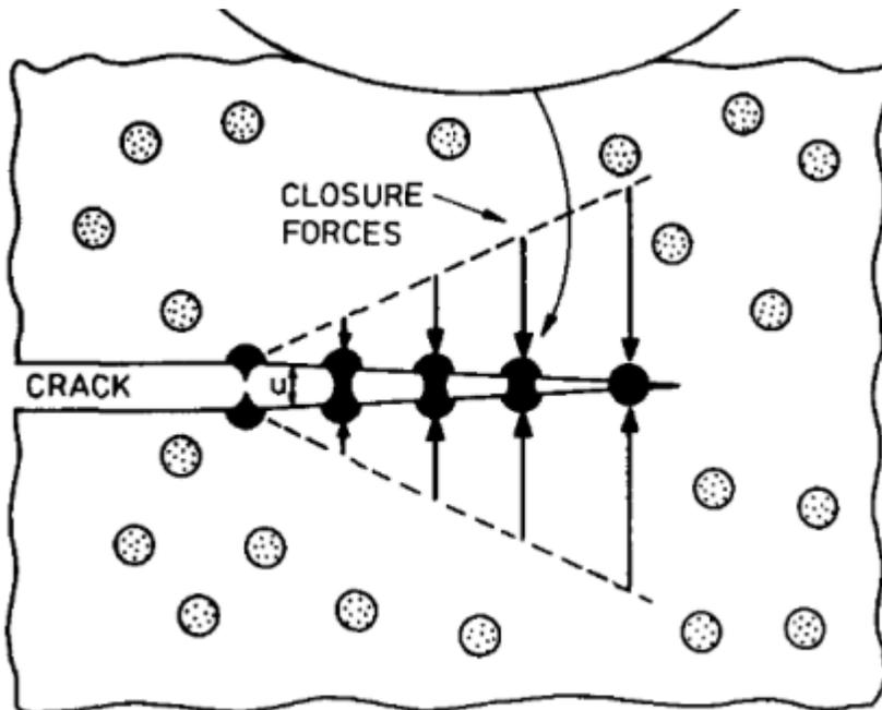
Fig. 1.4 demonstrates how particulate fibers are able to close cracks in ceramic composites by applying a closure force [4]
