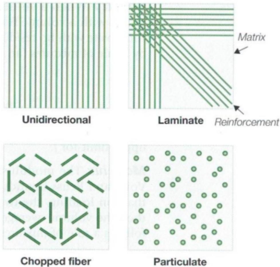
Fig. 1.2 showcases various fiber structures that can be used in ceramic composites [3]
