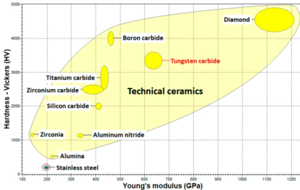
Fig. 2.1 shows an ashby chart that is used to determine the line of best fit to calculate hardness (Hv) based on Young's Modulus (GPa)
