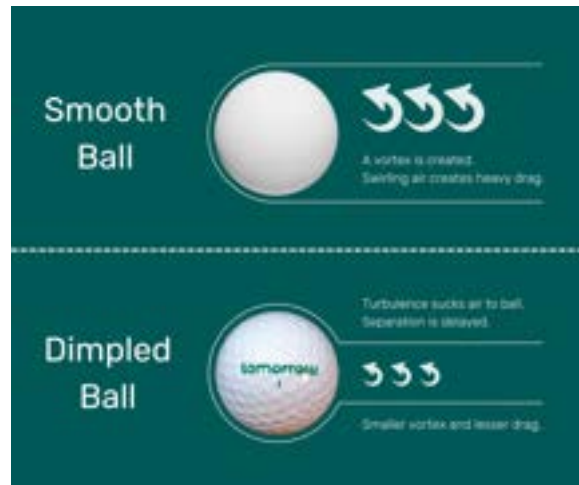
Figure C: Image explanation of golf ball dimples
