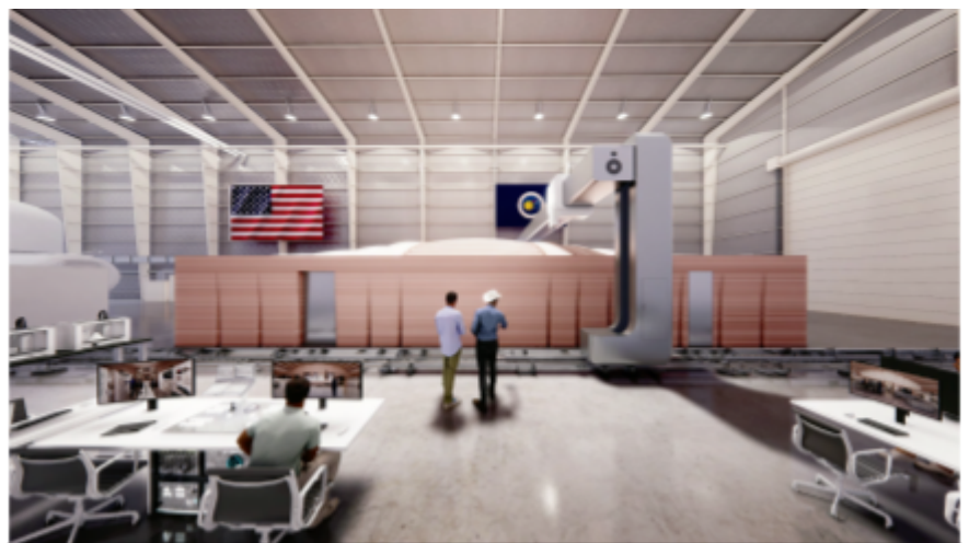
Figure 5. ICON 3D Prints the First Simulated Mars Surface Habitat for NASA Designed by Renowned Architecture Firm BIG-Bjarke Ingels Group (ICON, 2021).
