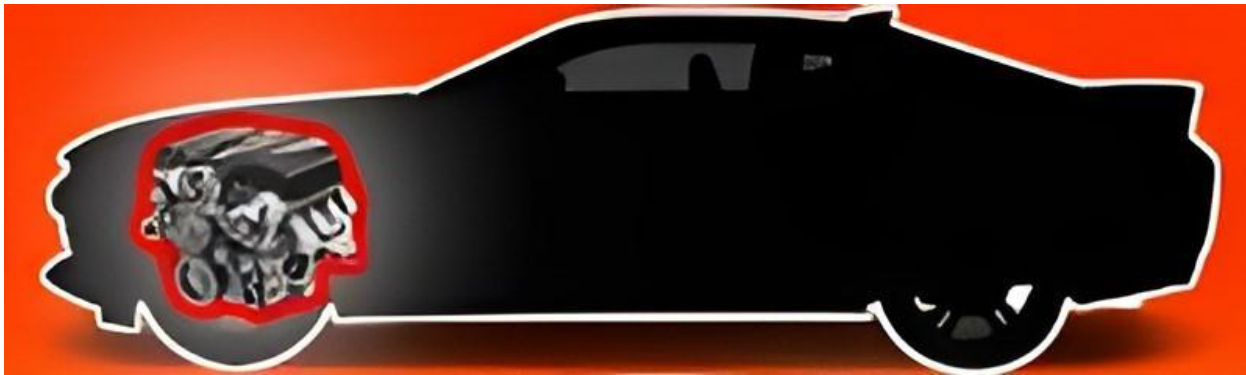
Figure 3 - A schematic that depicts that the engine is located in the front of the car for ICE vehicles. In most ICE-powered vehicles, the engine is placed at the front of the car. This allows the engine to be easily accessed and leads to better traction.
