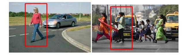
Both of the above images are examples of when the model correctly identifies and highlights a pedestrian on the street.
