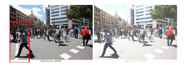
The accuracy after lowering the image brightness drops to 0.5 for images with pedestrians and 1.0 for images without. For example, in the following images, the pedestrians are undetected by the model when the brightness of the image is lower.
