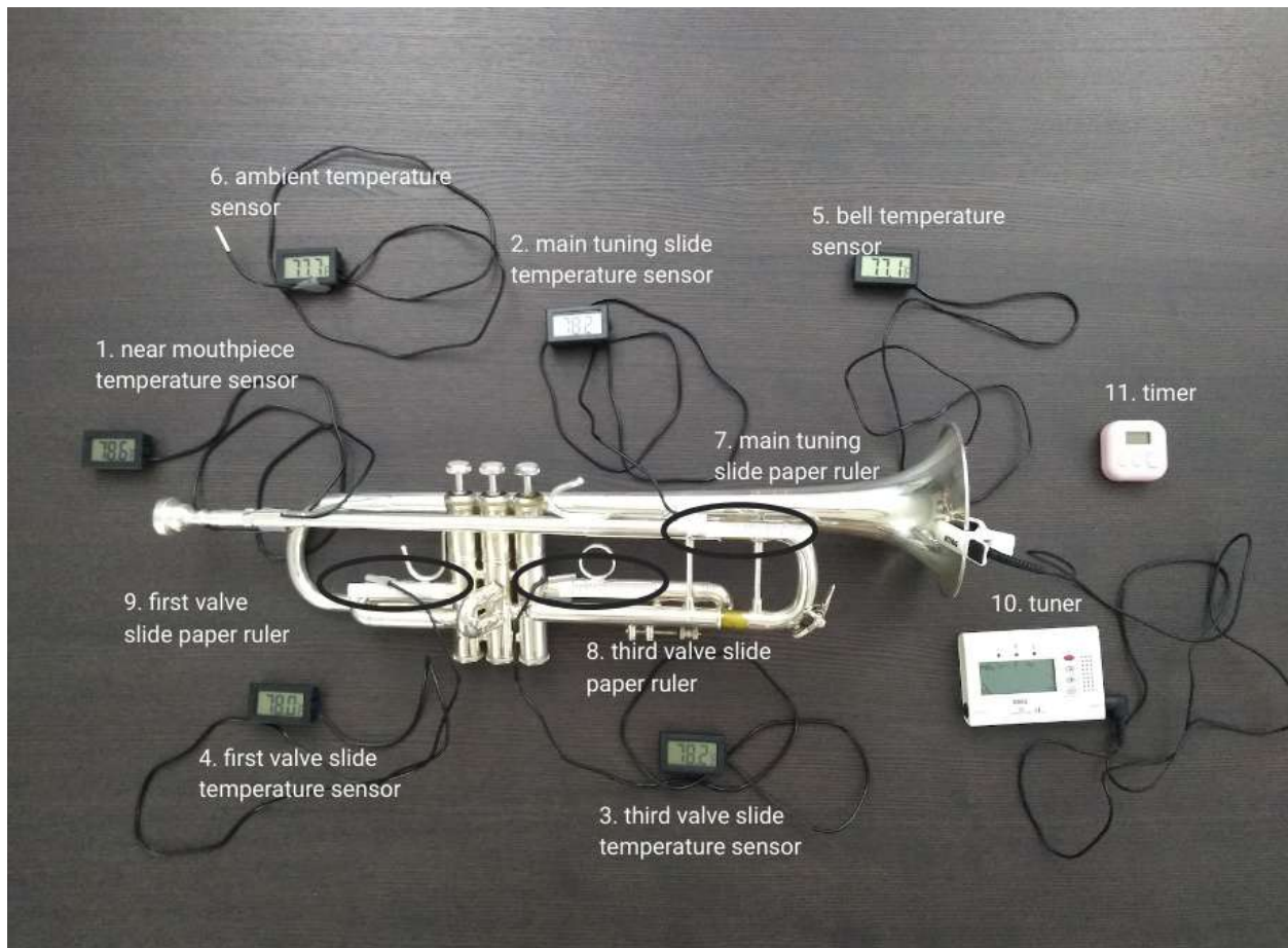
Figure 2. Experimental Setup used in this study. It consisted of 6 temperature sensors, three paper rulers, a trumpet, tuner, and timer. Five temperature sensors and three paper rulers were taped to the trumpet at respective locations labeled above.
