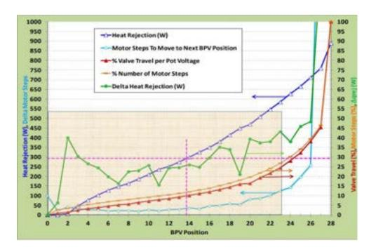
Figure 2: Heat Absorption from SWME. Increased water movement proportional to heat rejection
