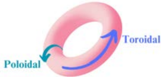
Figure 5. Poloidal and toroidal magnetic fields in a tokamak
