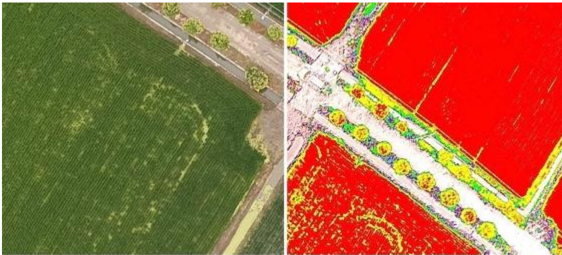
Figure 2: RGB VS. Multispectral Camera [13]
