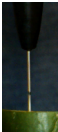
Figure 4: Example of a penetration test on a cucumber
