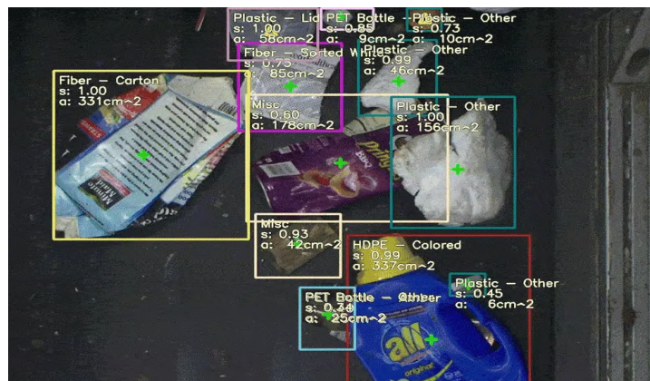
Figure 11: An AI object detection system automatically identifies and sorts trash to help reduce the amount of water pollution caused by improper disposal.
