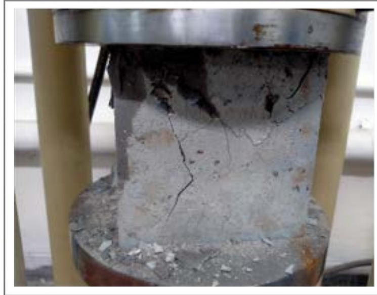
Fig. 7: Breaking point of concrete block on CTM
