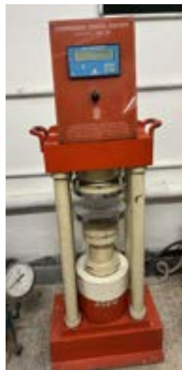
Fig. 6: Compression Testing Machine with a capacity of 2000 KN
