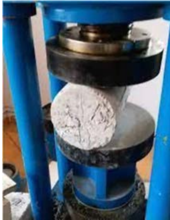
Fig. 8: Tensile strength test of cylindrical concrete block
