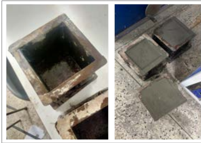
Fig. 5: Concrete samples being prepared for compression test
