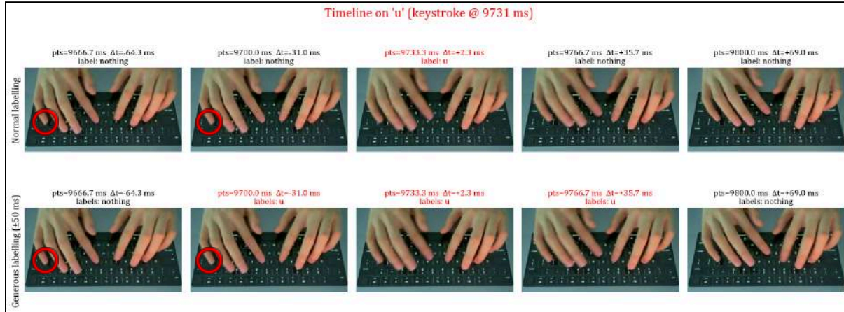
Figure 23b: This showcases a timeline on an ‘u’ keystroke, with timestamp of 9731ms. The first timeline shows normal labelling, while the second shows generous labelling. The red circles show where, by visual judgment, the actual keystroke could have occurred.
