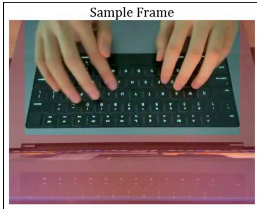
Figure 4: Shows a sample frame. The unnecessary pixel data is highlighted in red. This information is not important for the keystroke inference and just contributes additional noise.
