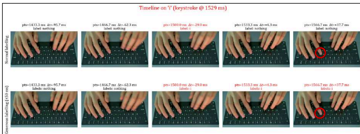
Figure 23a: This showcases a timeline on an 'i' keystroke, with timestamp of 1529ms. The first timeline shows normal labelling, while the second shows generous labelling. The red circle shows where, by visual judgment, the actual keystroke occurs.
