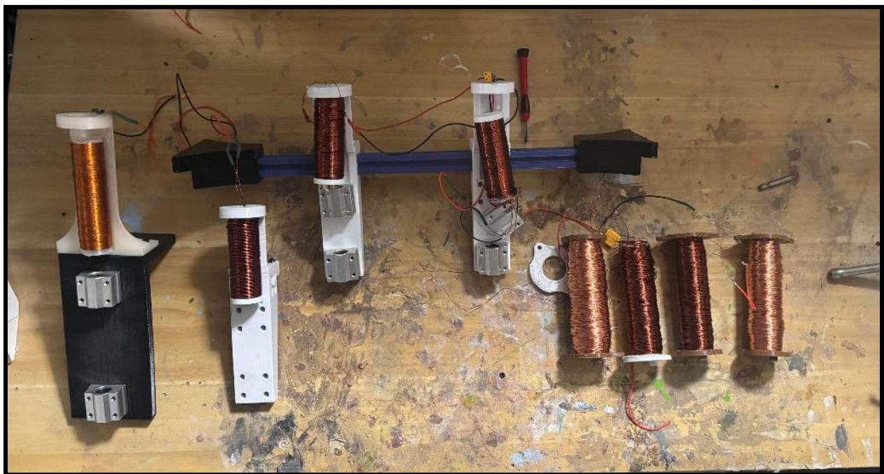
Photo 4: Depicted are the many failed attempts to create an effective coil, experimenting with different gauges and lengths of wire.
