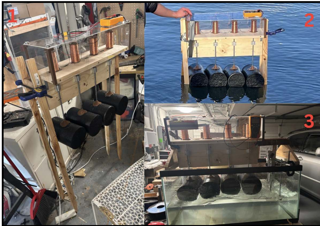
Figure 3: Section (1) displays the system integrated on top of wooden stakes that could be anchored into the ground. Section (2) shows the generator placed in San Francisco's Crane Cove to undergo testing. Section (3) depicts the same generator placed in the testing environment for a more convenient demonstration.
