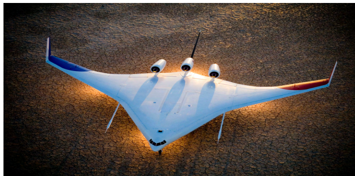
Figure 2: Commercial Blended Wing Body Design Depiction
