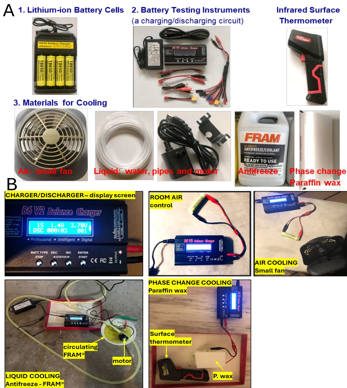
Figure 1. Materials shown in (A) were setup as shown in (B) using the various cooling methods and data
