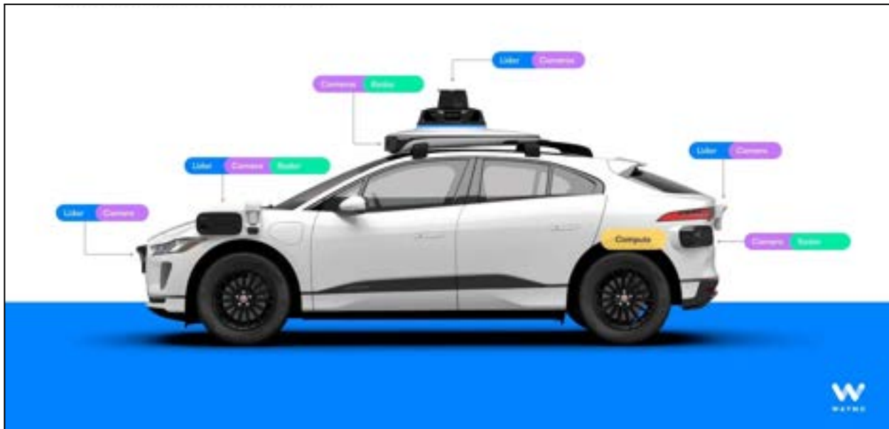
Figure 11. Indicates locations of LiDAR, radars, and cameras around the Waymo Jaguar I-PACE. [60]
