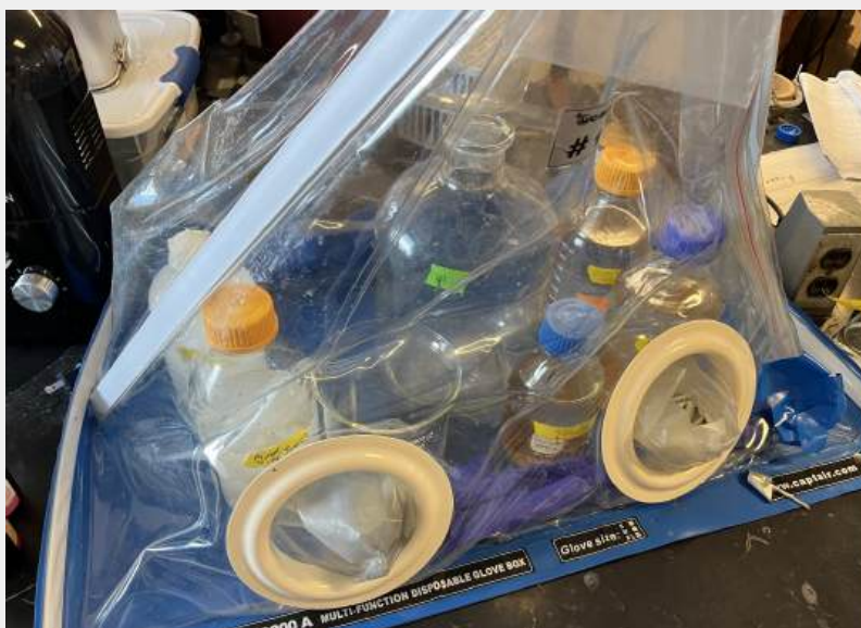
Figure 3: Glove box pumped with N_2 gas to prevent contact with oxygen. Old media bottle, new media bottle, and waste disposal bottle.
