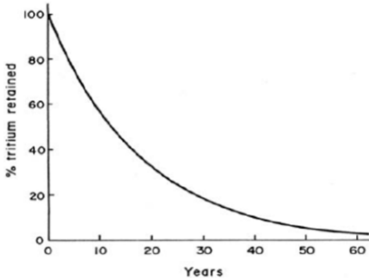
Figure 19: Radioactive decay curve of tritium from a test in Al-Shanafiya, Iraq (49)
