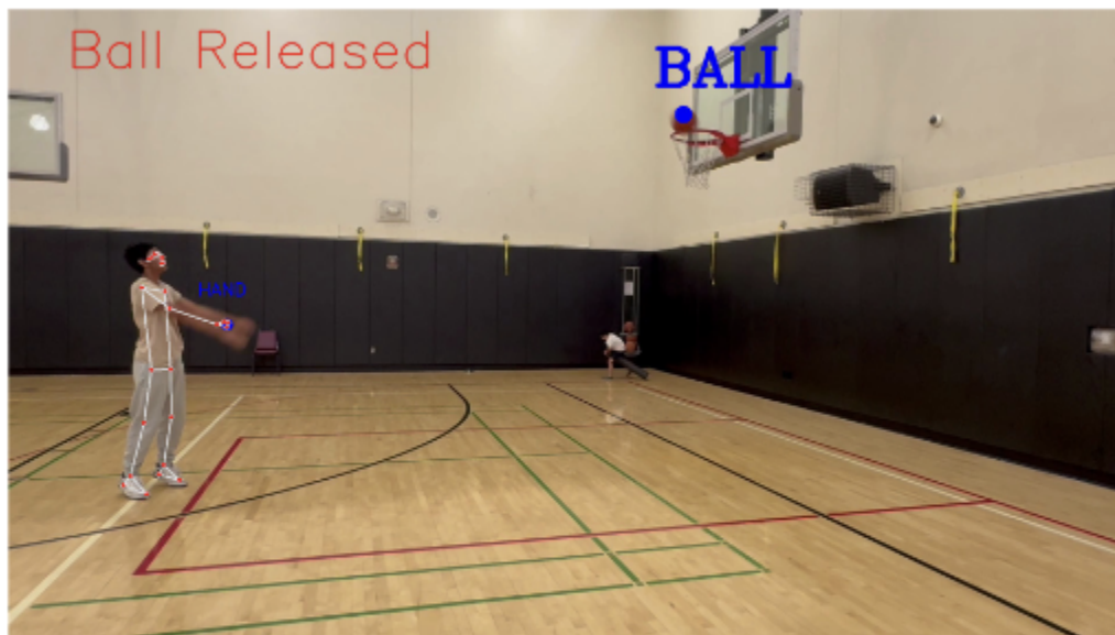
Fig. 1. We used an R-CNN pre-trained model to detect the ball right before it enters the basket. We utilize Mediapipe to detect the pose and hand features to ensure bodily features are not considered as the basketball.
