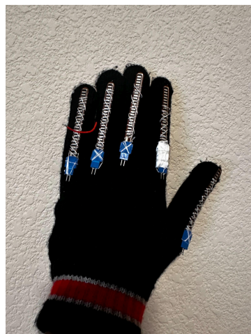
Figure 6. Glove with the flex sensors attached.
