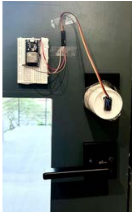
Figure 9. Setup of ESP32 and servo to complete the front door system
