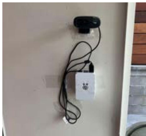
Figure 6. USB webcam connected to one of the available USB ports of the Raspberry Pi.
